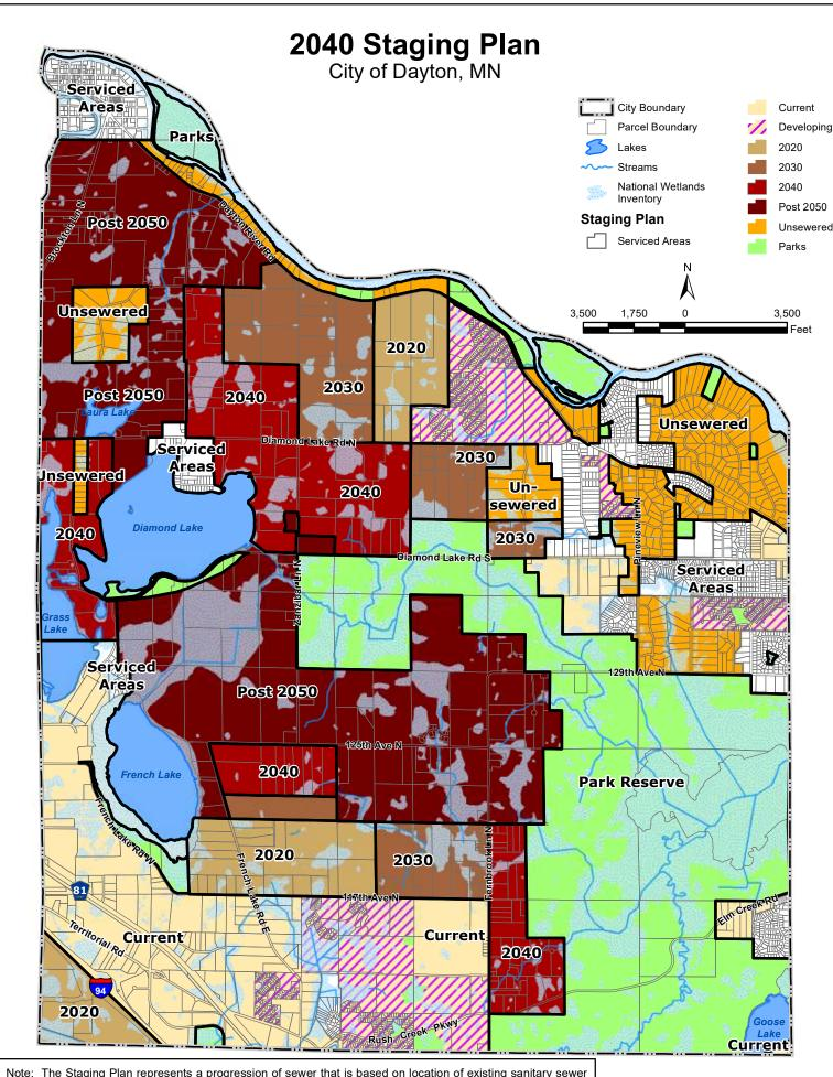
Note: The Staging Plan represents a progression of sewer that is based on location of existing sanitary sewer and anticipated extension as development progresses. The city does not commit to extensions occurring.
